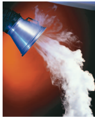
Standard hood design allows smoke bypass.
